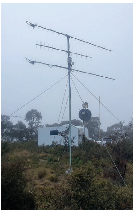
Fig.22 (left): a partial view of the (foggy) Field Day site showing some antennas, including two dishes and an equipment van. The top dish has a 24GHz amplifier and transverter behind it, while the lower dish contains preamps and an antenna for 1.2GHz - 10GHz.
