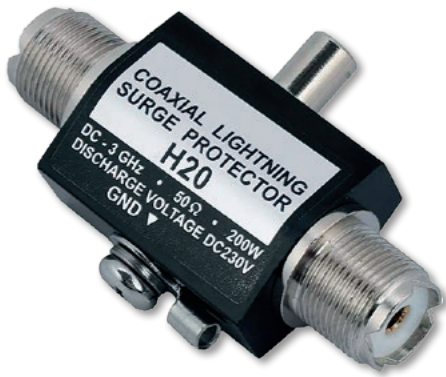
Fig.18: a lightning surge protector that can direct excessive charge buildup to the ground to minimise damage from a lightning strike.
