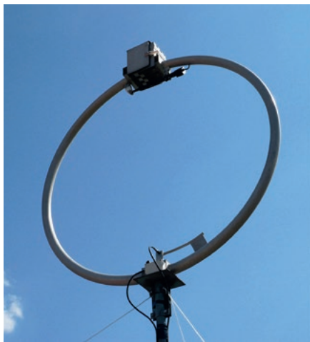
Fig.14: a magnetic loop antenna. Source: https://w.wiki/93Y4 (GNU FDL).
