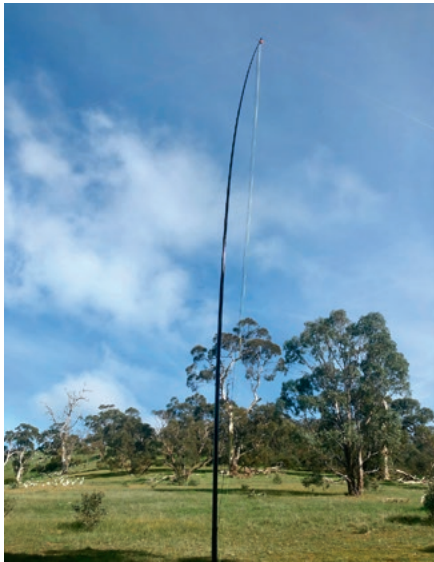
Fig.12 (left): a field-expedient vertical antenna supported by a squid pole.
